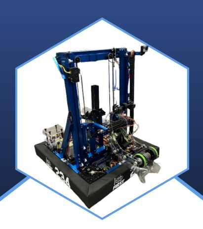
Our 2025 Robot was designed to have multi-mode autonomous. Our robot can load coral from the loading zone, and can load algae from the floor and from the reef. Our intake is also our output, allowing us to move the coral without a hand-off. We also have an in-frame climber that uses a winch and a magnet to climb on the lower level barge.
